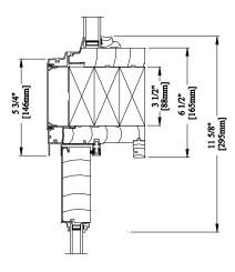
C - HORIZONTAL 3-1/2" [89mm] STACK SECTION (a)
