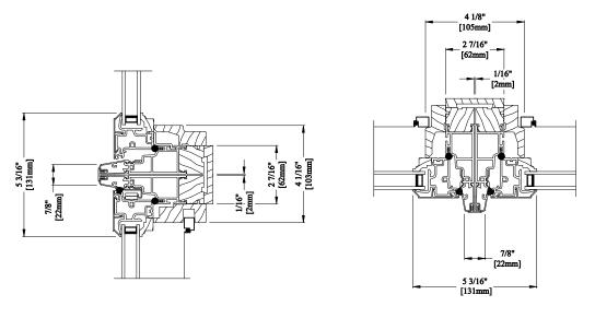
C - HORIZONTAL TIGHT STACK SECTION (a)
